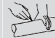
The spigot should be marked with a pencil line at a distance equivalent to the socket depth. Clean the surface within the marked area.
