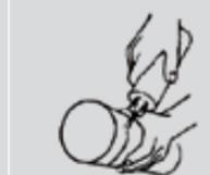
Apply lubricant on the external surface of the chamfered end of the pipe and on the rubber gasket.
