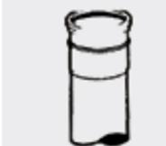
Check that the ring seal is in position in the housing.
