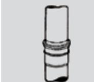
Withdraw the pipe until the mark is 12 mm away from the socket before fixing. This gap between the pipe end and the socket register is very essential for thermal expansion/contraction.
