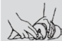
All burrs from the internal and external surfaces should be removed.
