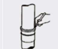
Push the pipe fully into the socket and mark the pipe depth in the socket with marker.
