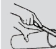
Chamfer the end of the pipe. Remove all burrs, dust and dirt.
