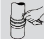
Remove the excess solvent cement and hold the joint firmly in position for 30 seconds to dry.
