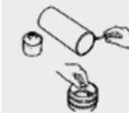
Apply uniform coat of solvent cement on the external surface of the pipe and a lighter coat on the internal surface of the fitting.
